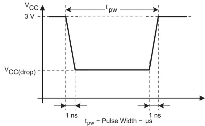
Figure 11. V<sub>CC(drop)</sub> Level With a Square Voltage Drop to Generate a POR/Brownout Signal
