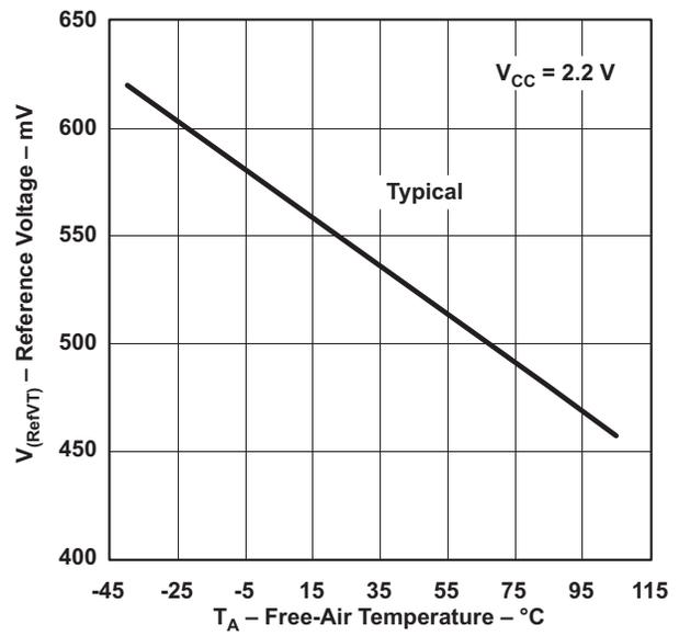
Figure 15.  $V_{(RefVT)}$  vs Temperature,  $V_{CC} = 2.2\text{ V}$
