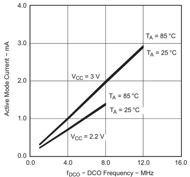
Figure 3. Active Mode Current vs DCO Frequency
