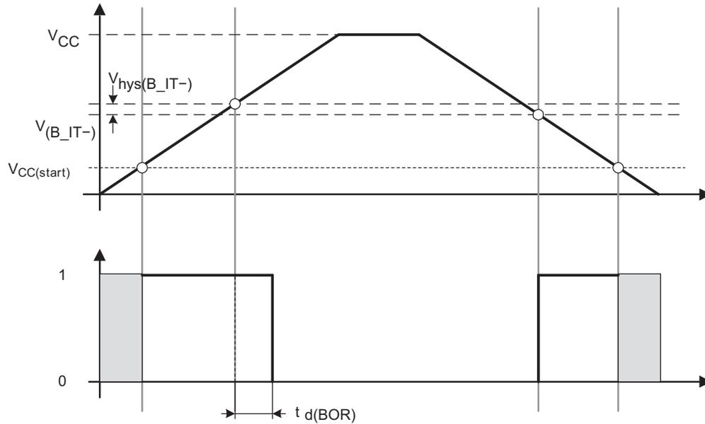
Figure 10. POR/Brownout Reset (BOR) vs Supply Voltage
