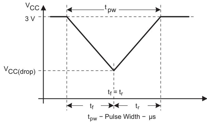
Figure 12. V<sub>CC(drop)</sub> Level With a Triangle Voltage Drop to Generate a POR/Brownout Signal
