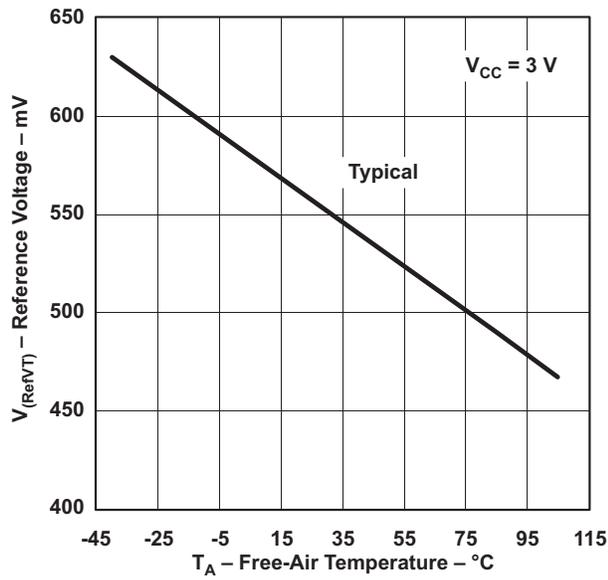
Figure 14.  $V_{(RefVT)}$  vs Temperature,  $V_{CC} = 3\text{ V}$
